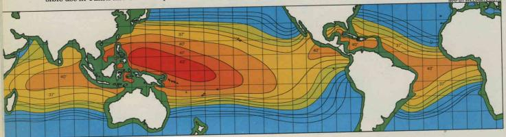
At the best sites for OTEC plants, colored red on the map above, the surface water is 43 degrees Fahrenheit warmer than the water 3,000 feet below. But the plants could also use cooler waters, shown in shades of orange, where the temperature difference is usually at least 37 degrees
